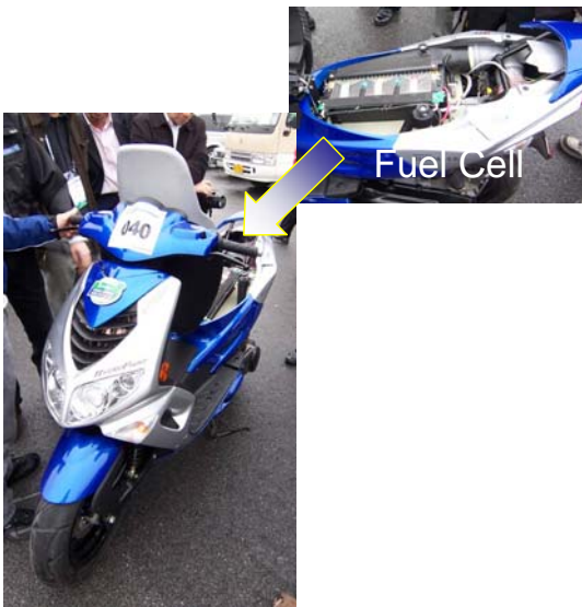
Figure 8: Daimler demonstrated a fuel-cell-powered scooter at the 2007 Challenge Bibendum in Shanghai, the epicenter of China's shift from 2- to 4-wheeled personal transport.
